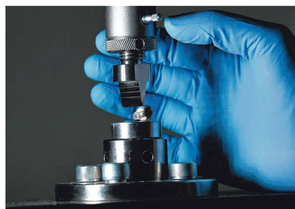
9 A test being conducted on the force required to remove dental fillings by shear stress on a tooth. This is done by simulating the biting action, which will cause the filling to fall off.
