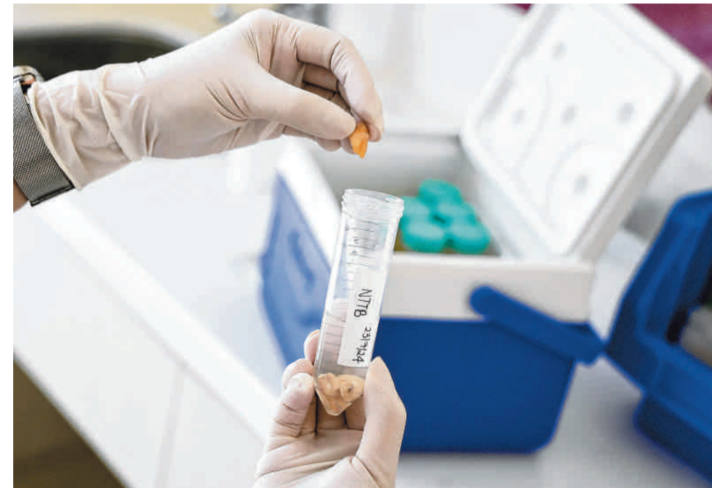
4 Each tooth is soaked in an alcohol solution to decontaminate it before it is transferred into a test tube with highly purified water. The test tube is then placed in a box.
